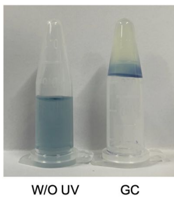
Figure S1. Characterization of hydrogel. Photograph of hydrogel prepared from 10 wt% of PEG-DA and 1 wt% of I2959 with or without UV irradiation (6W) for 15 min.
